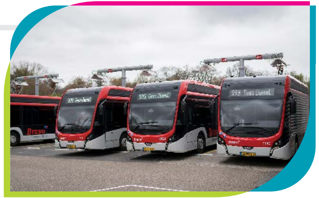
The buses during the charging and pre-heating of the battery
