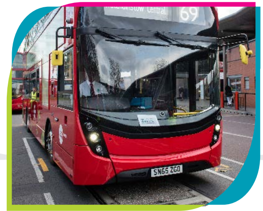
Bus positioning for charging
